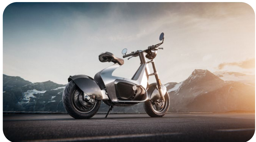
Origami-Inspired STILRIDE bends a sheet of steel to form a swanlike electric motorcycle.
