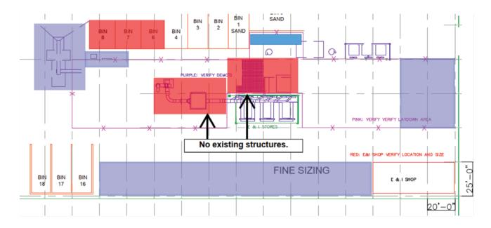
electronic components. It is not unheard of for expensive pieces of equipment to "walk away" from a jobsite! Fig. 4 is an example of a laydown yard imposed over an existing floor plan. All red areas represented "claimed" areas, whereas all purple areas represented space available for equipment. The laydown yard drawing should be updated and distributed regularly to the project team.
