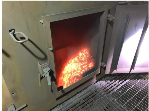
Material inlet situation at the kiln outlet at Grange Resources Port Latta Plant: From 2020 an AUMUND Steel Plate Conveyor type KZB-H will transport the iron ore pellets at a temperature of up to 750°C to the cooler. (Photo AUMUND)
